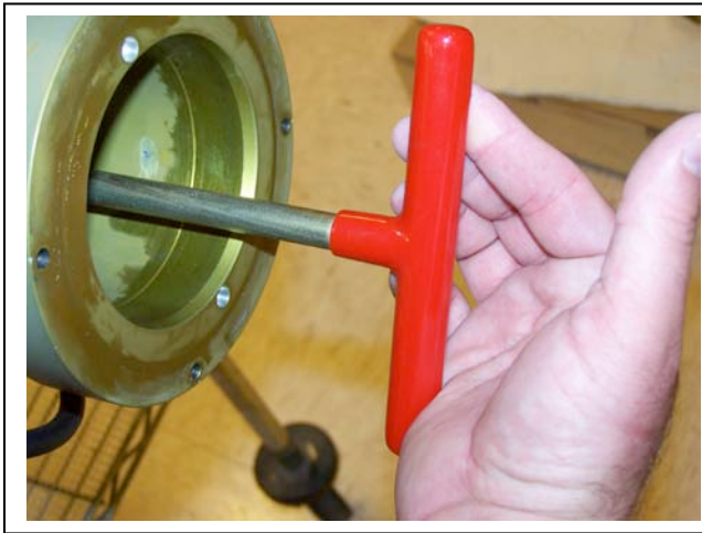
Figure H-6: Removing DVS Connection Plate
