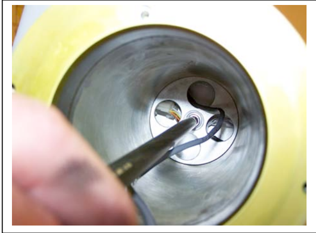
Figure H-13: Tightening Connection Plate
