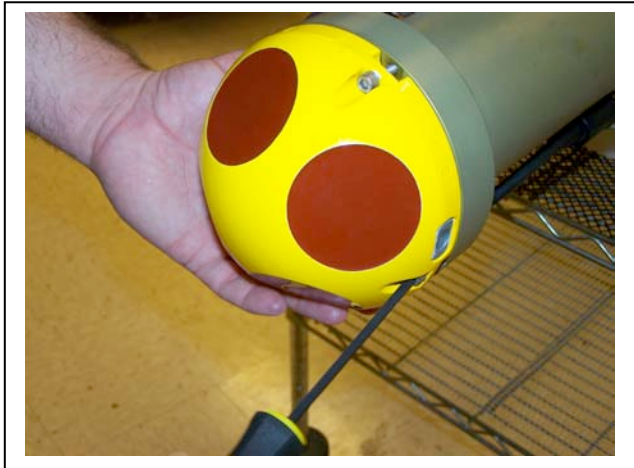
Figure H-15: Reattaching DVS Sensor Head
